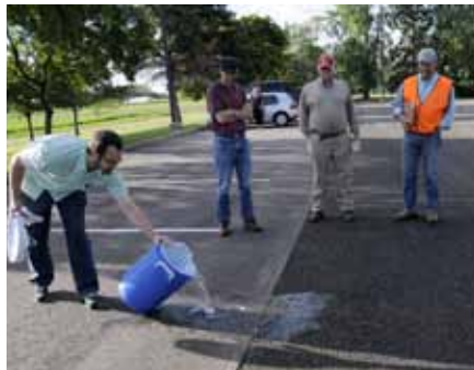
Demonstration of pervious asphalt near Larpenteur
